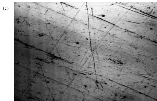
Fig. 5(a-b): (a-b) 3-D surface roughness R_a after EPDAP (c) Electron Microscope photograph at 100X of EPDAP surface
