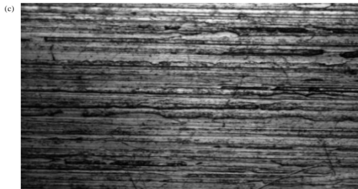
Fig. 4(a-b): (a-b) 3-D surface roughness R_a of ground surface and (c) Electron microscope photograph at 100X of ground surface
