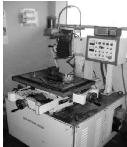
Fig. 3: Sparkonics Micro-EDM machine, (Brass Electrode dia 0.4 mm), Courtesy- Covai EDM, Coimbatore
