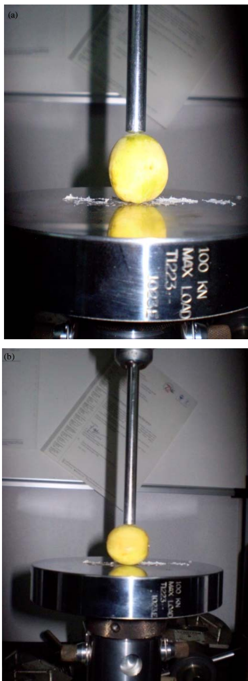
Fig. 4(a-b): Two different loading positions of Jatropha curcas L. fruits
