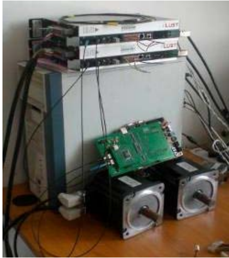
Fig. 14: Scenario for Sercos II communication system verification
