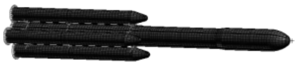
Fig. 2: Finite element model of rocket-spacecraft coupling system
