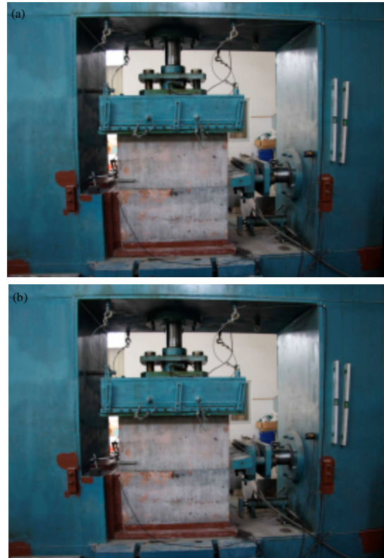
Fig.7: Integrative direct shear apparatus (a) Big device and (b) Small device
