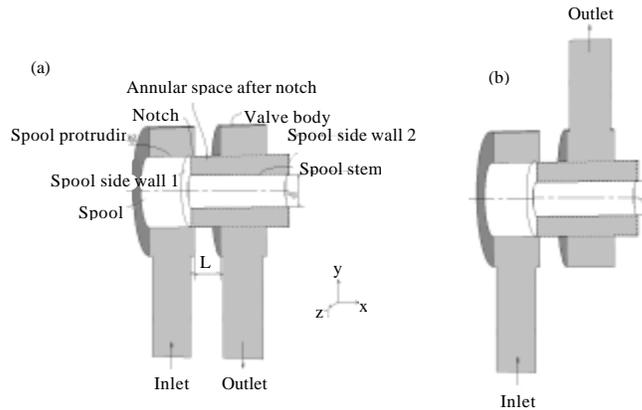
Fig. 1(a-b): 3D model of the valve, (a) Same side of Inlet and Outlet passage and (b) Opposite of Inlet and Outlet passage
