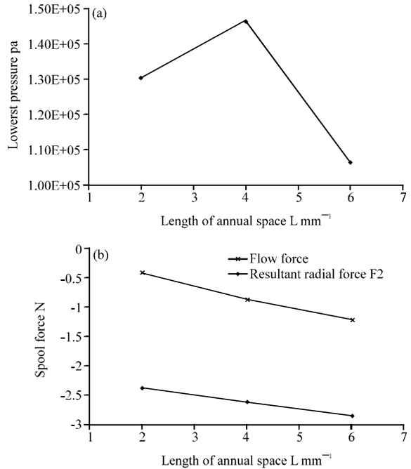
Fig. 11(a-b): Lowest pressure value and forces on the spool relation to the length, (a) Lowest pressure value and (b) Forces on the spool
