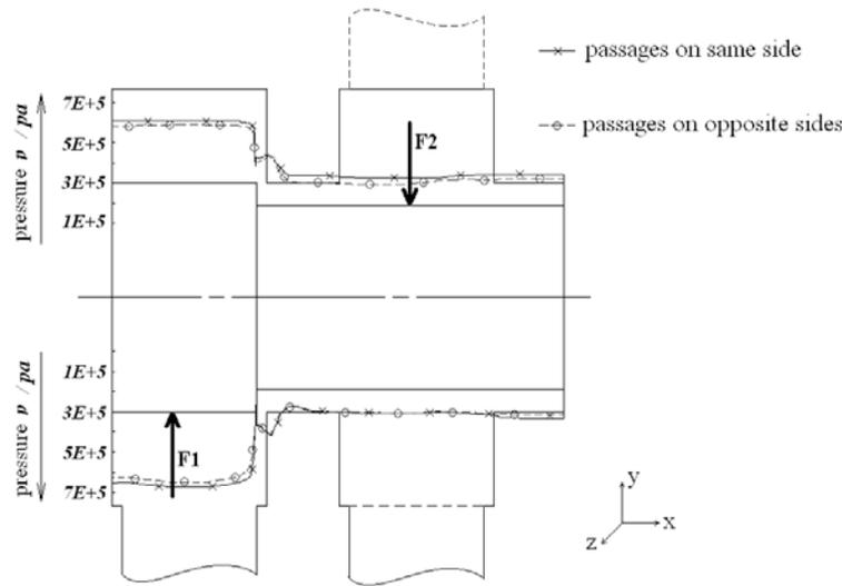
Fig. 12: Comparison of the axial pressure distributions
