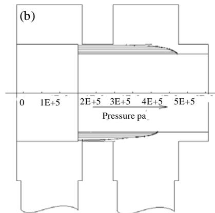
Fig. 8(a-b): Pressure distribution on the side walls of the spool, (a) Pressure distribution on side wall 1 and 2, (b) Pressure distribution on side wall 1
