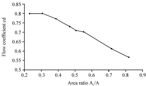
Fig. 6: Flow coefficient of the valve
