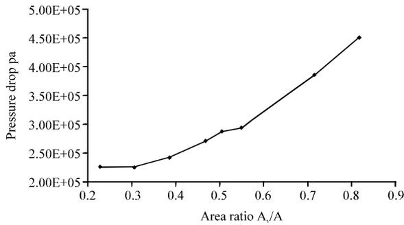
Fig. 5: Pressure drop of the valve
