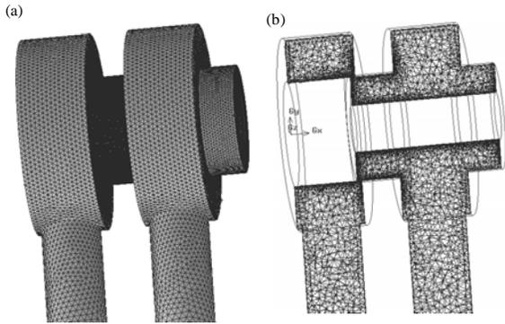
Fig. 2(a-b): Computational grid of the valve, (a) Computational grid of the whole valve and (b) Meshing on the symmetry plane
