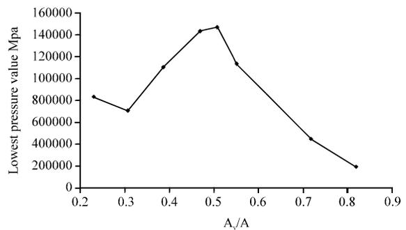
Fig. 4: Relationship between the lowest pressures and area ratio
