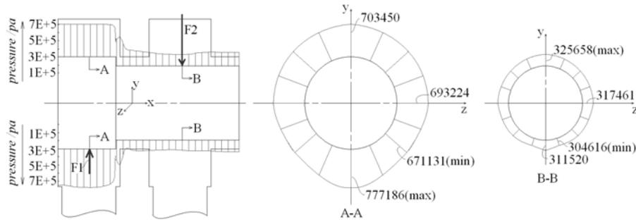
Fig. 9: X-axial and radial pressure distributions on the spool
