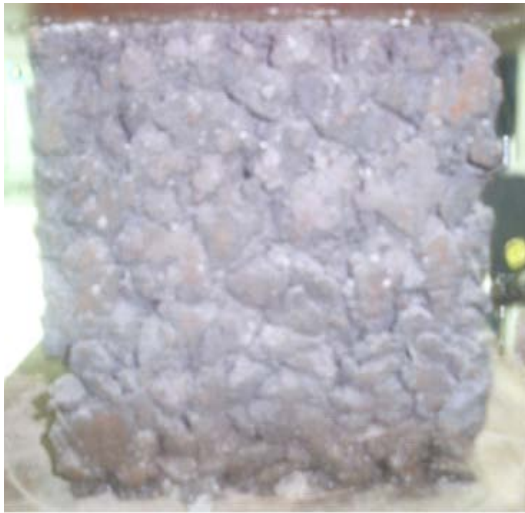
Fig. 3: Cracks of the EPC specimen
