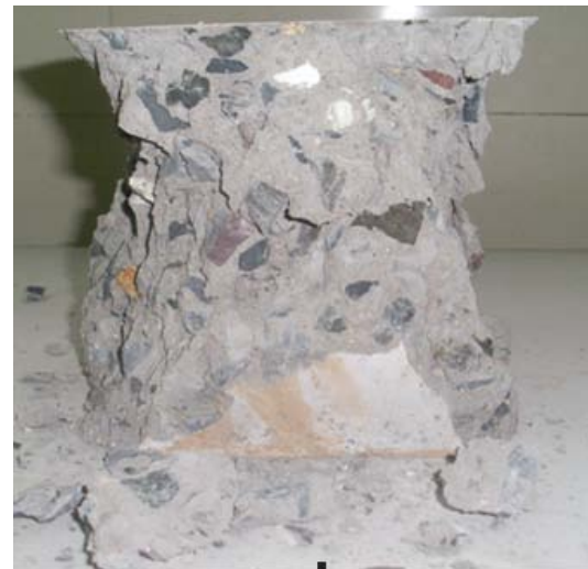
Fig. 2: Vertical pyramid type failure of TC specimen
