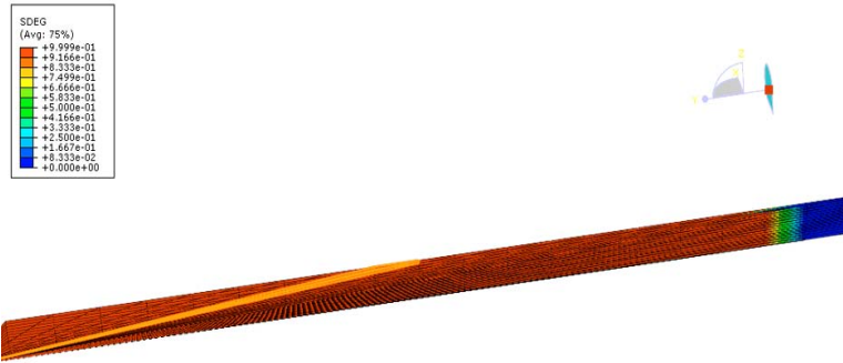
Fig. 7: Crack length of azimuth angle is 0°
