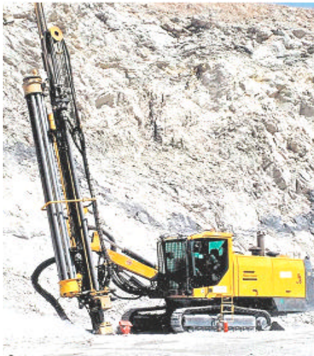
Fig. 1: Hydraulic drill working
