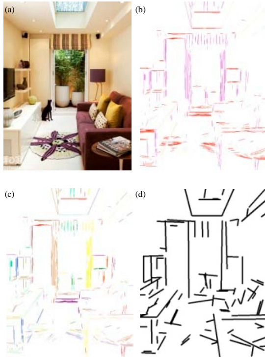
Fig. 6(a-d): Experiment procedure with interior scene image used. (a) Input original image; (b) Direction clustering result from (a); (c) Distance cluster result from (b); (d) Final clustering result from (c)
