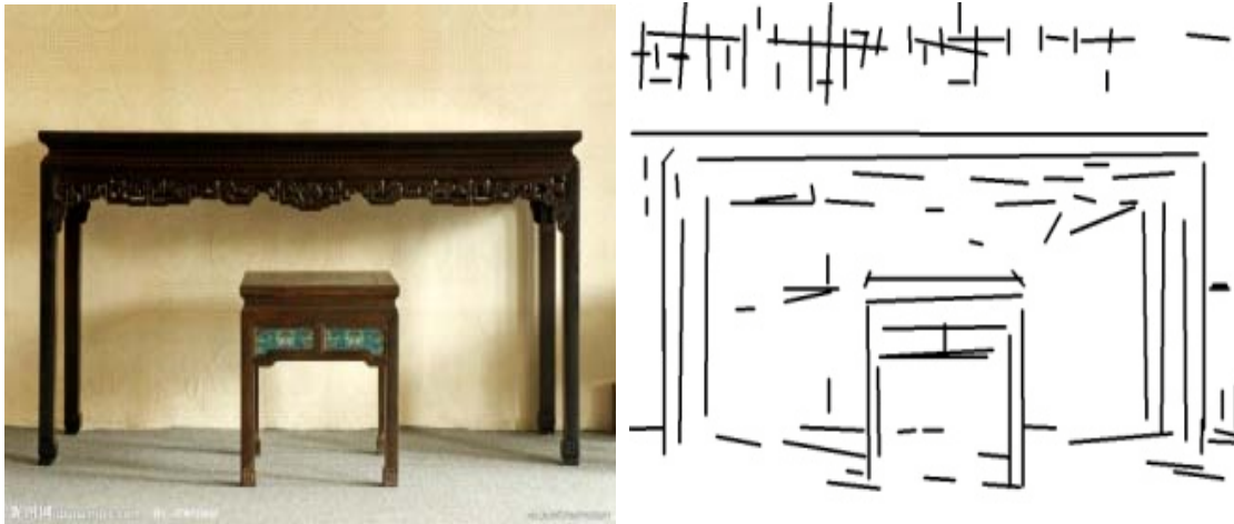
Fig. 7: Experiment results of several test image about real scene, (a), (b) and (c) give three examples to illustrate the right-column final clustered line segments from the left-column original image, respectively
