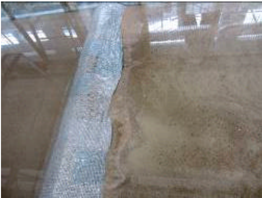
Fig. 13: Photos after scouring under the condition of 5 cm drop height before and after the dam
