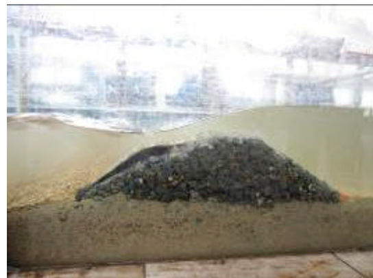
Fig. 8: Photos of the ballast dam body with concrete and grouted rag collapse (a) Water damage firstly occurred where permeability rate is larger (b) Whole dam body damaged
