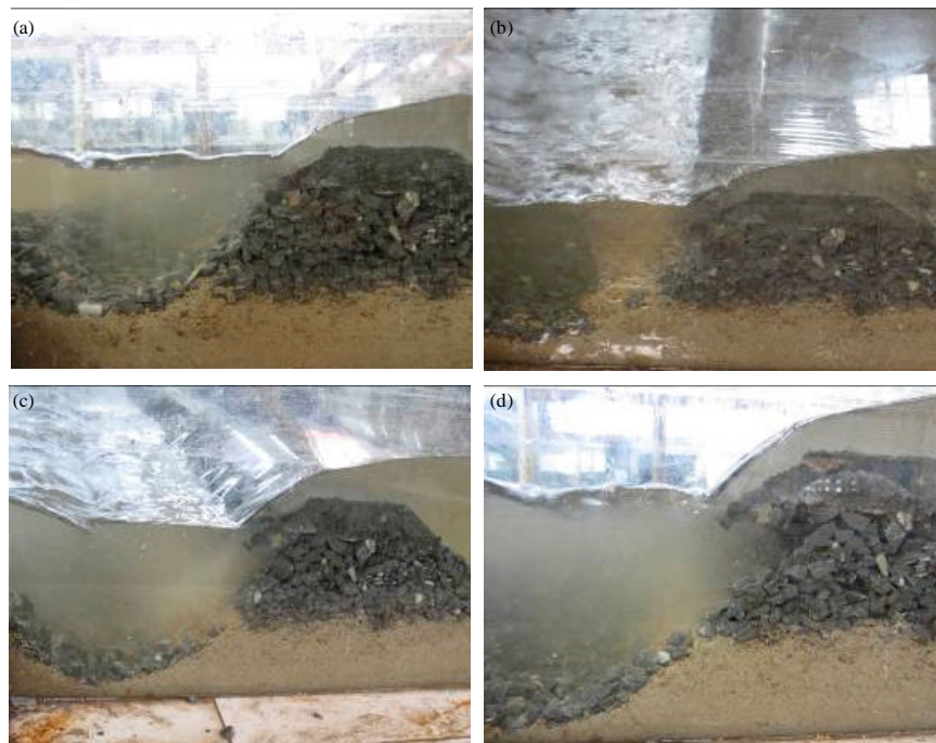
Fig. 7(a-b): Photos of the ballast dam body with concrete and grouted rag water damage process (a) Water head before and behind the spur dyke is 4.5 cm (b) Water head before and behind the spur dyke is 5.5 cm (c) Water head before and behind the spur dyke is 6.1 cm and (d) Water head before and behind the spur dyke is 7.1 cm
