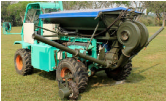
Fig. 1: Variable rate technology fertilizer applicator on the prime mover
