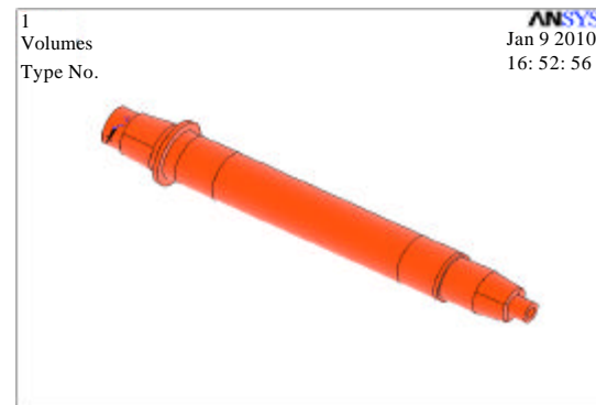
Fig. 1: Spindle finite element model diagram
