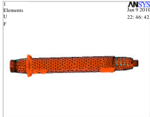
Fig. 4: Spindle limited load figure
