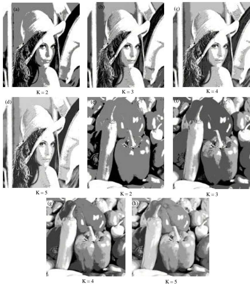
Fig. 6(a-h): Segmented images using threshold values found by BA algorithm (a and e) used two thresholds, (b and f) used three thresholds, (c and g) used four thresholds and (d and h) used five thresholds
