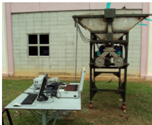
Fig. 1: Metering system test rig for the VRT fertilizer applicator
