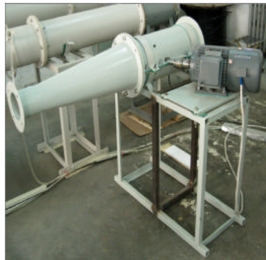
Fig. 1: Physical map of axial-flow fire-fighting fan test equipment
