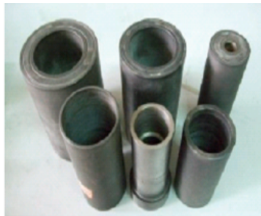
Fig. 2: A set of molds for metal rubber
