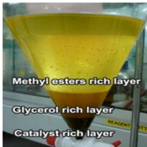
Fig. 1: Three separated layers after transesterification of WCO
