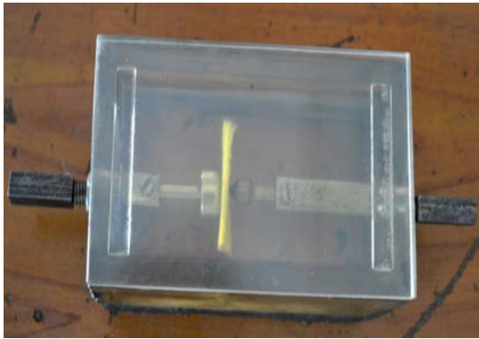
Fig. 4: Sample test specimen from 11 kV XPLE cable for HFHV test
