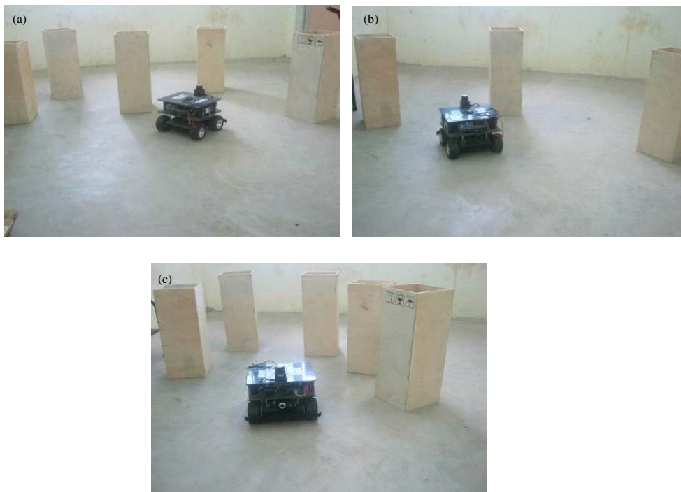
Fig. 3(a-c): (a) Mobile robot encountering a cluttered environment, (b) Mobile robot encountering a sparse environment and (c) Mobile robot encountering a closed environment
