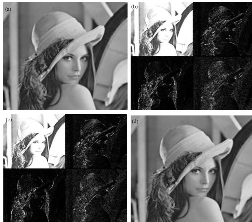
Fig. 4(a-d): Lena image, (a) Original image, (b) DWT 1 st level image, (c) IDWT 1 st level image and (d) Reconstructed image
