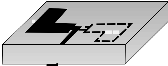
Fig. 5: Sample of a biplane dipole antenna in Z-topology fed at its centre by a microstrip transmission line
