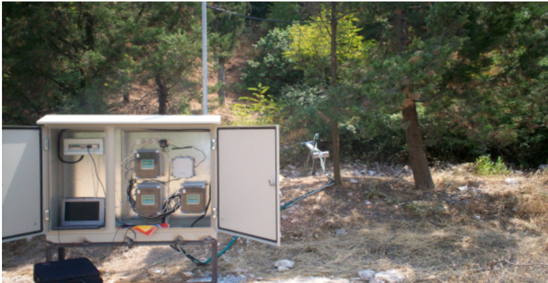
Fig. 2: Experimental set up for the on-line measurement of pH, redox potential and temperature. Both sensors and data logger unit are shown
