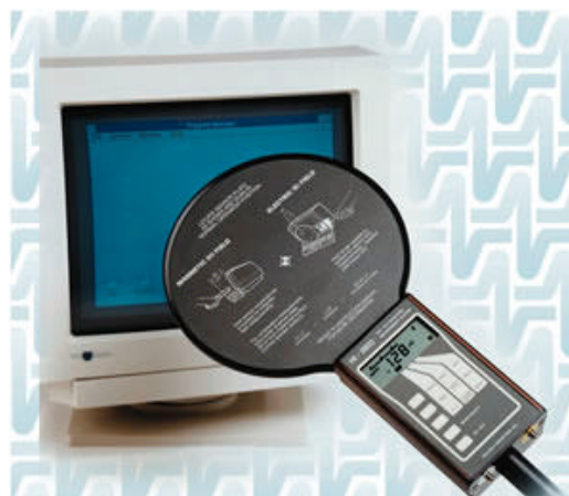
Fig. 1: A view of the holiday magnetic field meter (HI-3603) used in this study
