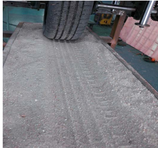
Fig. 4: Slip rate of 15.1% during traction test
