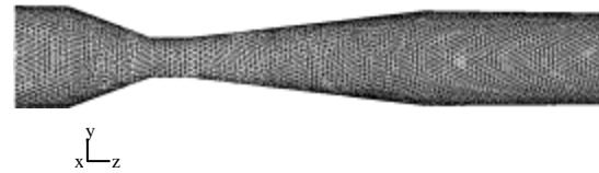
Fig. 3: Meshed geometry of venturi meter for standard venturi design 2A
