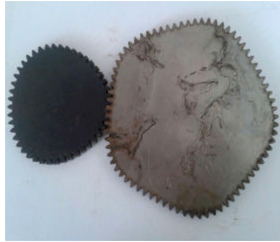
Fig. 6: Physical structure of elliptical gears
