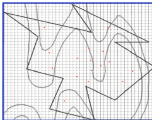
Fig. 1: Contour generation in the regular region that contains the irregular region (The black line indicates the boundary of the irregular region, red dots the discrete data, the blue line the smallest rectangular region and the gray curves the contours generated)
