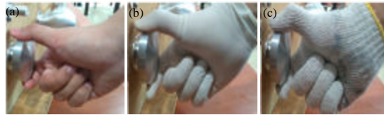
Fig. 3(a-c): Examples of different tactile sensations used when pinching a cylindrical knob (a) Cylindrical knob pinched with bare hands, (b) Cylindrical knob pinched with increased sensation and (c) Cylindrical knob pinched with reduced sensation
