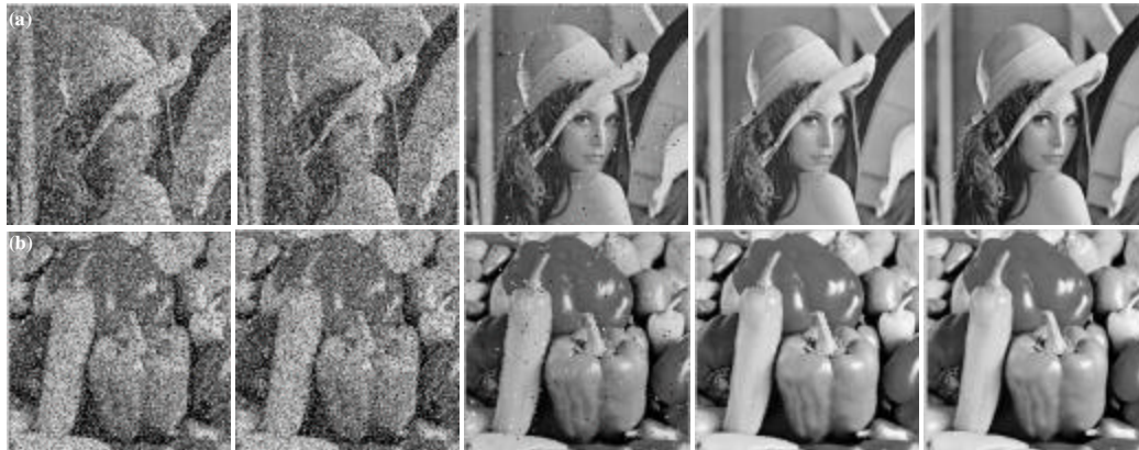
Fig. 3(a-b): Simulation results of different algorithms for 30% noise added to (a) Lena image: Noisy image, median filter, AMF, DBA, proposed approach and (b) Pepper image, noisy image median filter, AMF, DBA, proposed approach
