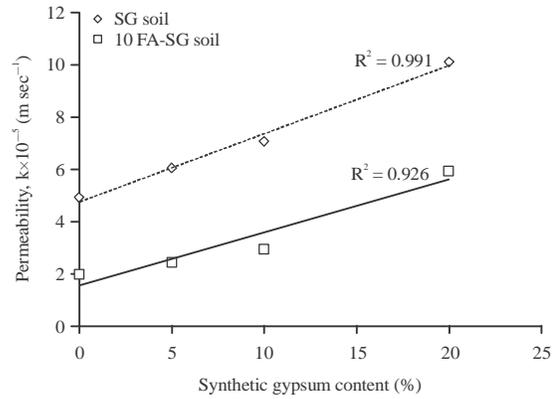
Fig. 5: Permeability of SG and 10 FA-SG soils
