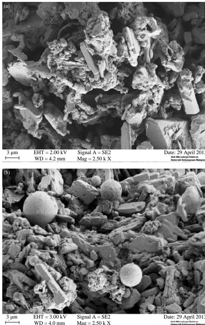
Fig. 1(a-b): Scanning electron microscope photographs of at 2.5 K magnification (a) Peat soil treated with synthetic gypsum (seen as elongate shapes) and (b) Peat soil treated with 10% fly ash (sphere shape) and synthetic gypsum
