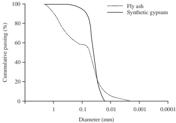
Fig. 2: Particle size distribution of additive materials used
