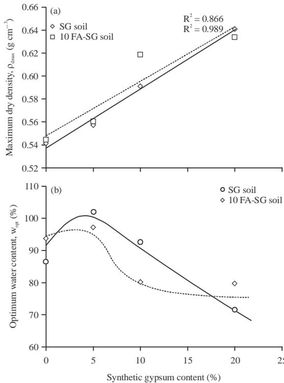
Fig. 4(a-b): (a) Maximum dry density,  $\rho_{dmax}$  values and (b) Optimum water content,  $w_{opt}$  against synthetic gypsum contents for SG and 10 FA-SG soils
