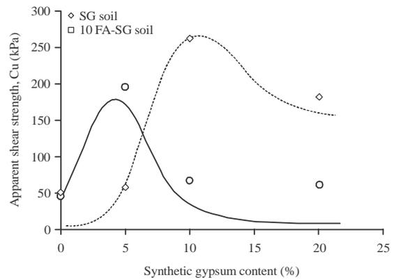
Fig. 6: Shear strength against synthetic gypsum contents of SG and 10 FA-SG soils
