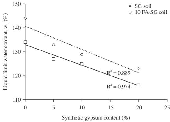
Fig. 3: Atterberg limit,  $w_L$  values against synthetic gypsum contents for SG and 10 FA-SG soils
