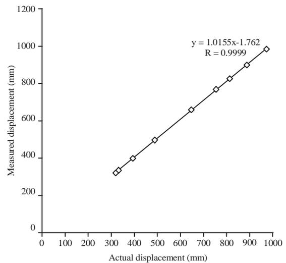
Fig. 28: Regression line for the sensors integration measurements
