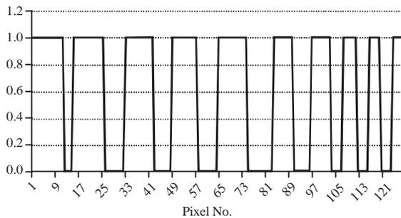
Fig. 22: Stripes image after thresholding process
