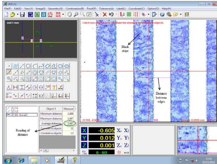
Fig. 15: Measurement of stripes width
