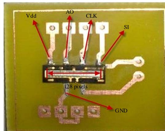
Fig. 3: Linescan sensor circuit
