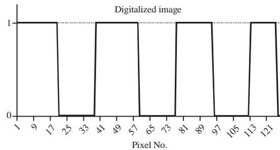
Fig. 20: Stripes image after thresholding process
