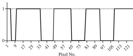
Fig. 26: Binary values based on thresholding process
