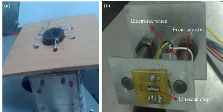
Fig. 1(a-b): (a) Outer components of the module and (b) Inner components of the module
