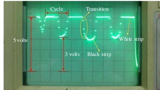
Fig. 12: Image of stripes as seen on the oscilloscope
