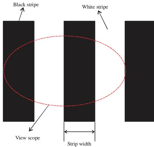
Fig. 4: View scope of linescan sensor
