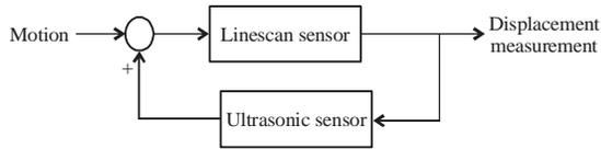
Fig. 10: An ultrasonic sensor is a feedback sensor for linescan sensor
