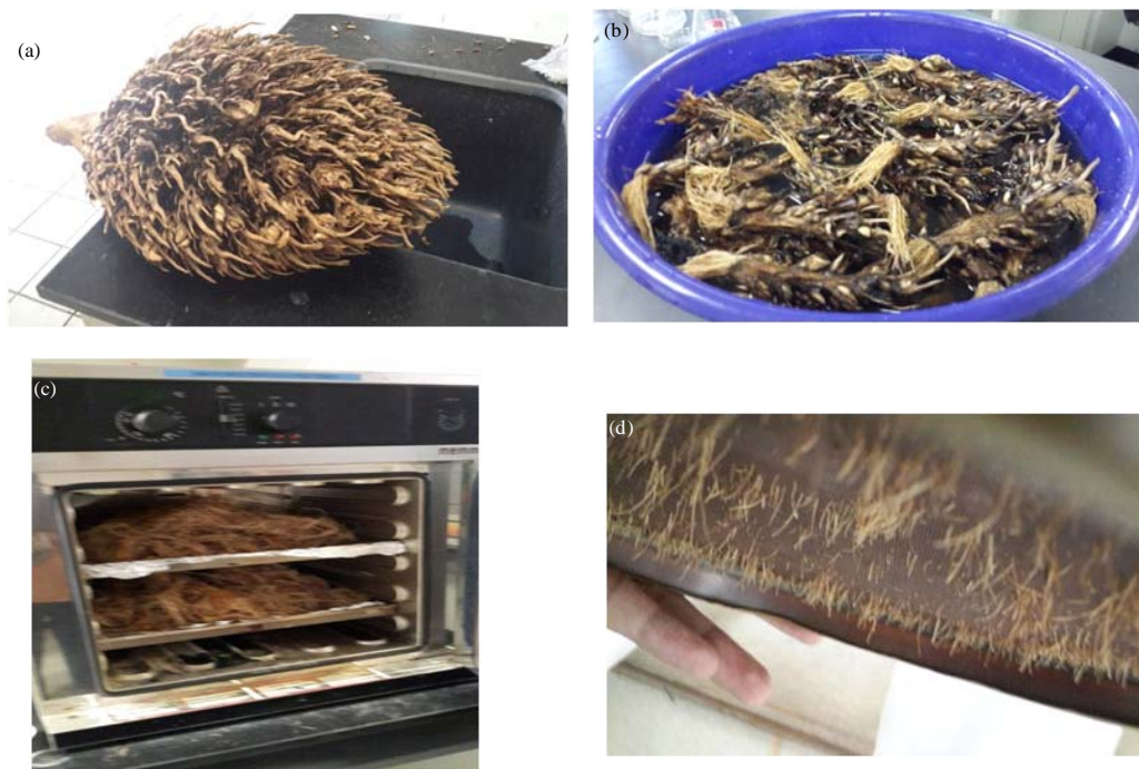
Fig. 1(a-d): (a) Obtained empty fruit bunch, (b) Washing with distilled water, (c) Drying in an oven at 130°C and (d) Sieving process
