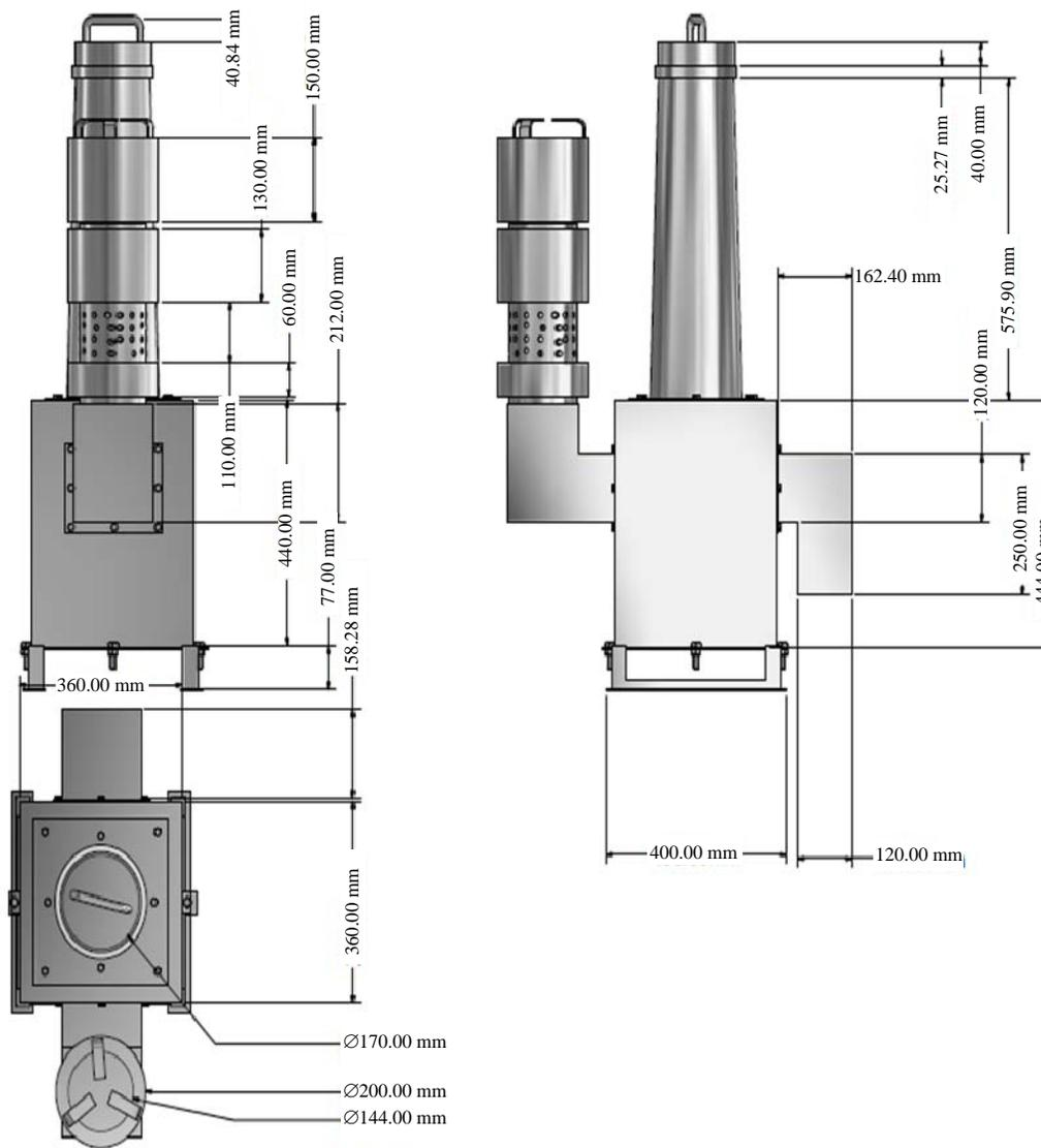
Fig. 3: First angle projection of the cross-draft gasifier stove
