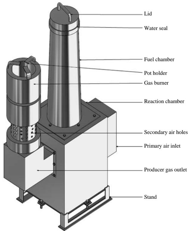
Fig. 1: 3-dimensional view of the cross-draft gasifier
