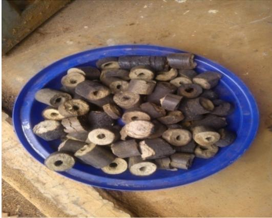
Fig. 4: Fuels used in the gasifier stove (rice husk briquette)
