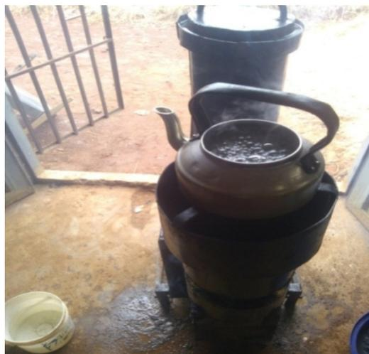
Fig. 8: Gasifier stove under water boiling taste
