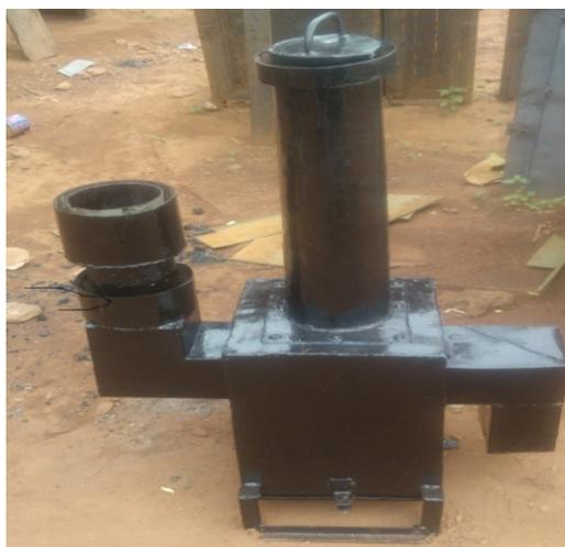
Fig. 7: Finished gasifier stove without pot stand
