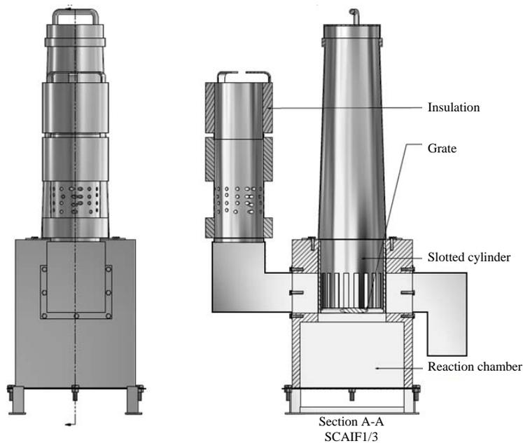
Fig. 2: Sectional view of the cross-draft gasifier stove
