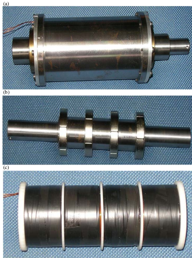
Fig. 11(a-c): Fabricated linear motor, mover and coil with coil casing, (a) Fabricated linear motor, (b) Shaft and permanent magnet assembly and (c) Coil and coil casing
