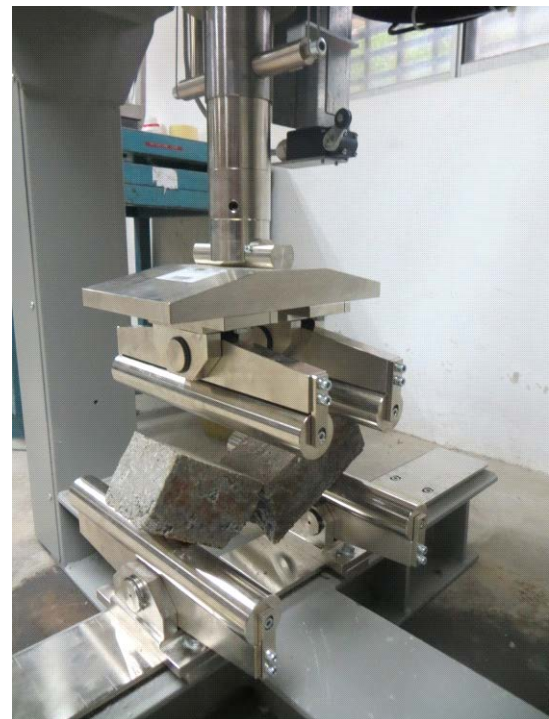
Fig. 5: Flexural strength testing setup
