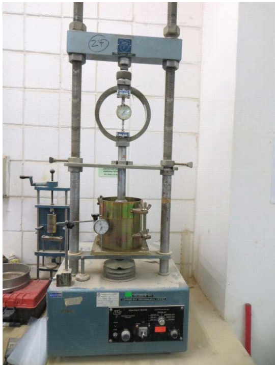
Fig. 6: California bearing ratio testing setup
