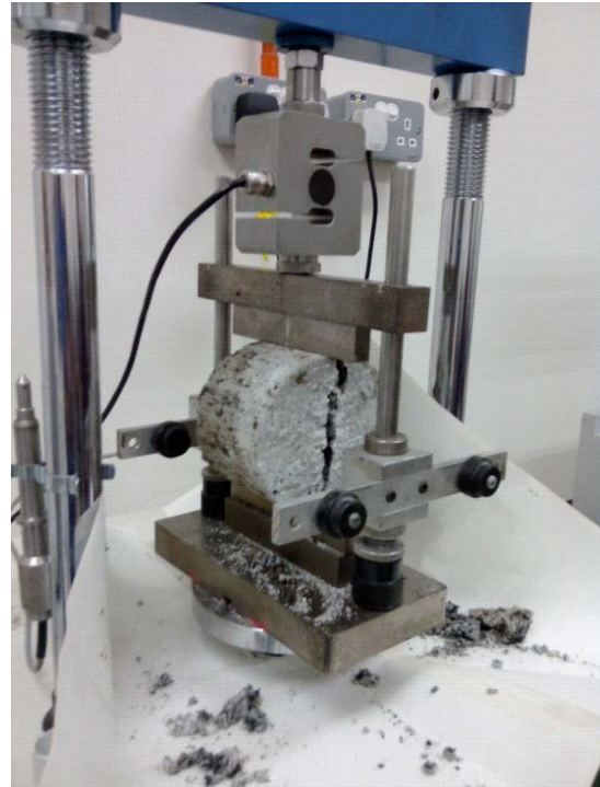
Fig. 3: Indirect tensile strength testing setup
