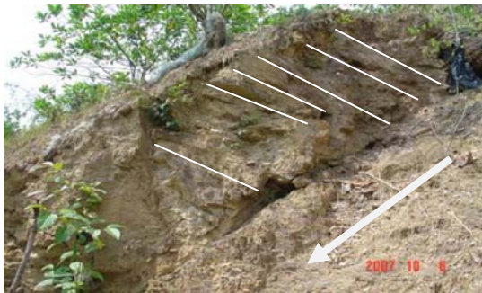
Fig. 7: Slope face dips to the east and the bedding plane dips to westward direction
