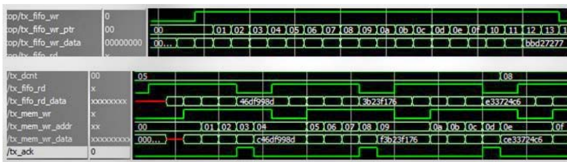
Fig. 7: Data writing to FIFO and reading from FIFO and then writing to memory
