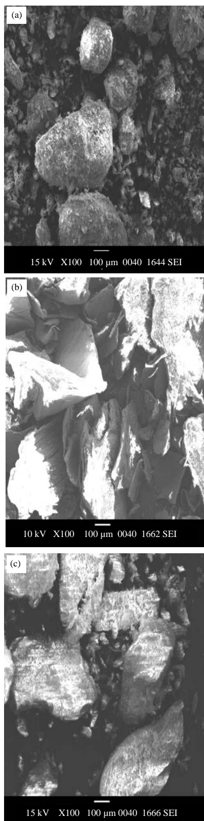
Fig. 3(a-c): SEM images of (a) Commercial chitosan, (b) Shrimp chitosan and (c) Crayfish chitosan
