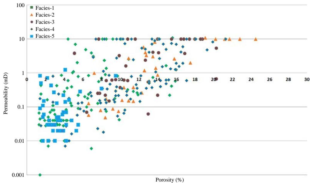
Fig. 9: Cross plot between porosity and permeability. Facies 5 represents minimum permeability of 1 mD, while facies 1-4 permeability is up to 10 mD
