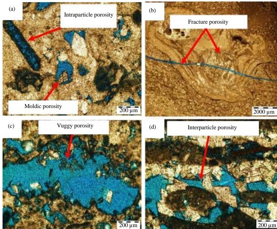
Fig. 8(a-d): Photomicrograph representing different types of porosity, (a) Intraparticle and moldic porosity, (b) Fracture porosity, (c) Vuggy porosity and (d) Interparticle porosity and partial filling of dolomite, dolomite cement filling pore spaces and the rate of dolomitization increase with time in well A and B, offshore Sarawak, Malaysia
