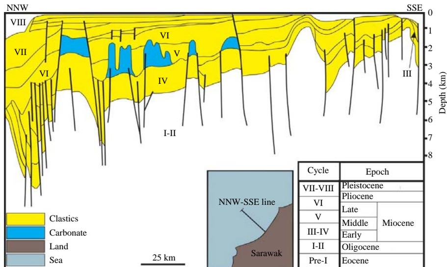
Fig. 3: Offshore Sarawak's structural sketch showing the boundaries of Central Luconia-a sector with numerous isolated carbonate platforms-in the Luconia province. Source: Janjuhah *et al.*<sup>62</sup>
