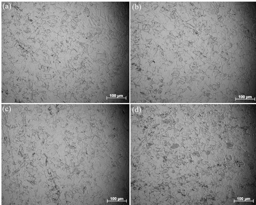
Fig. 4(a-d): Micrograph of austenite grain boundaries under different heat treatment conditions (a) 1173 K, 30 sec, (b) 1173 K, 60 sec, (c) 1173 K, 120 sec and (d) 1173 K, 240 sec
