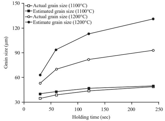
Fig. 3: Actual grain size vs. estimated grain size for different holding time
