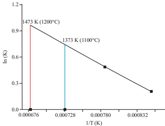
Fig. 2: Growth rate constant as a function of the reciprocal of the process temperature
