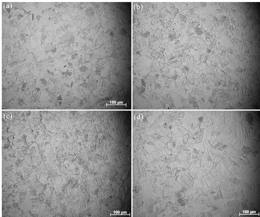
Fig. 5(a-d): Micrograph of austenite grain boundaries under different heat treatment conditions (a) 1273 K, 30 sec, (b) 1273 K, 60 sec, (c) 1273 K, 120 sec and (d) 1273 K, 240 sec
