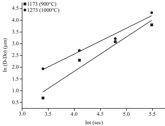
Fig. 1: Logarithmic plots of the grain size vs. the holding time after annealing at the annealing temperatures of 1173 K and 1273 K
