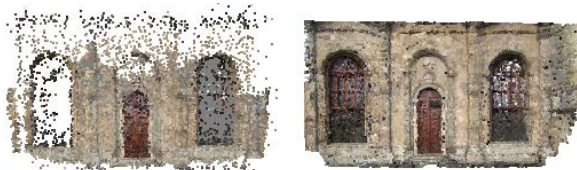
Fig. 2: Sparse (12587 points) and dense (680912 points) point cloud measurement data
