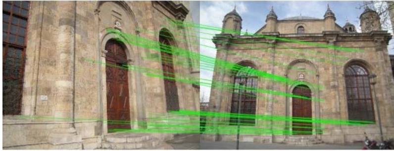
Fig. 11: Automatic matching results of the images that have a different scale and point of view angles (SIFT)
