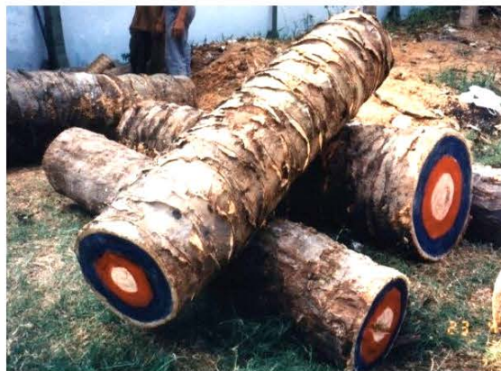
Fig. 1: Logs of matured oil palm stem used for experiment material. Note: The end of logs were colored differently, representing one-third of log's radius, to help in identifying the original positions of the resulting lumbers had been cut from
