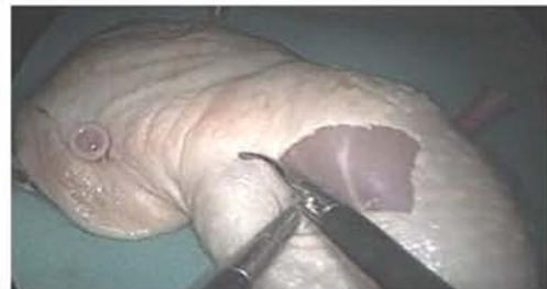
Fig. 4: Task 2, Endoscopic scissors to trail a pattern drawn on the skin of a raw chicken leg
