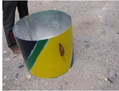
Fig. 1: The container used for DEW test (60 cm (height) ×60 cm (diameter))
