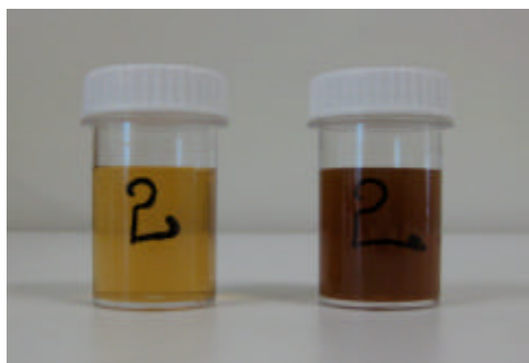
Fig. 1: Colour change of S. agardhii extracts containing silver before and after synthesis of silver nanoparticles
