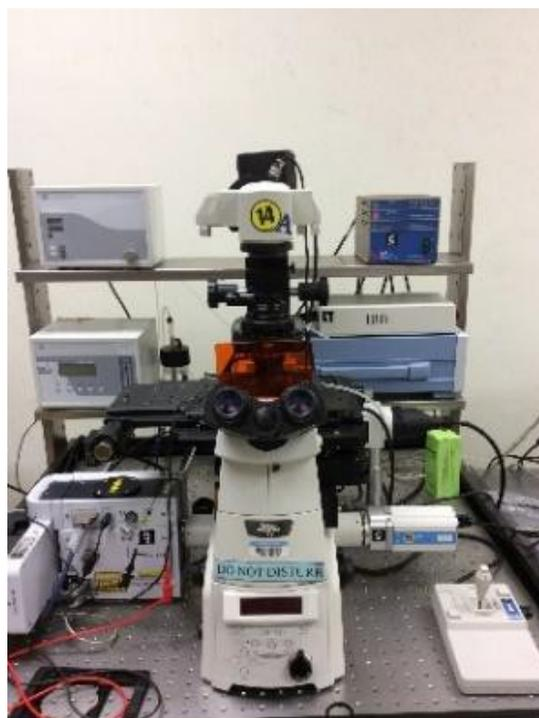
Fig. 4: Nikon inverted microscope (Ti series)
