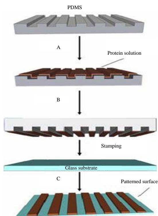
Fig. 2: Process flow schematic of microcontact printing method
