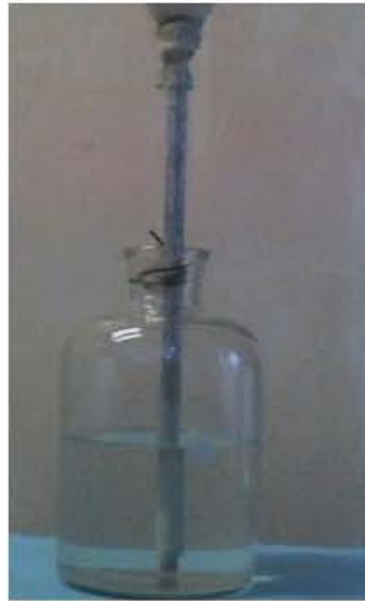
Fig. 2: Collection chamber fitted with metal stand (Mag: x0.45)
