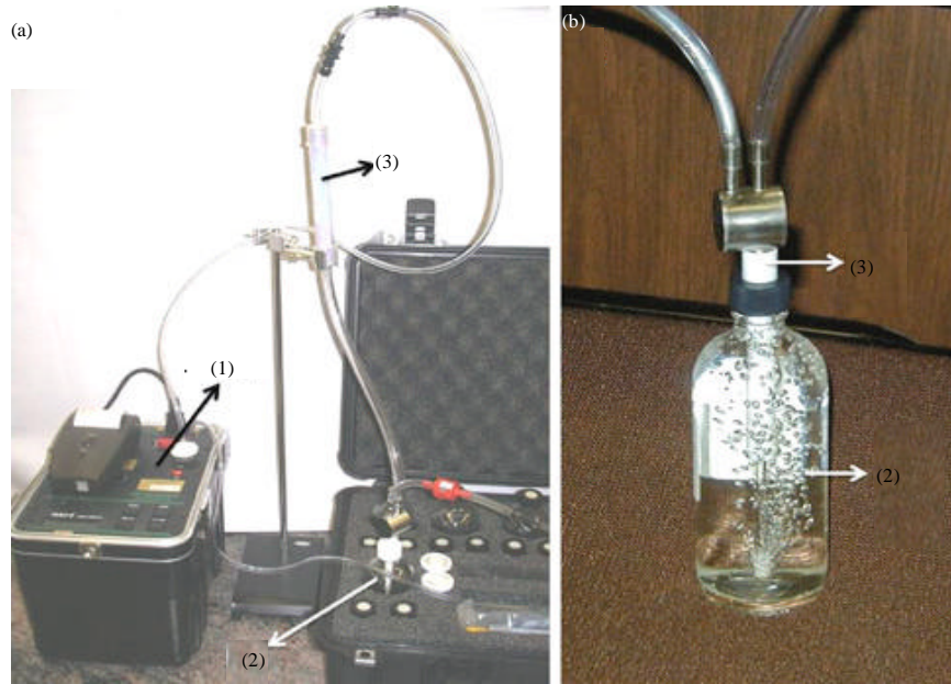
Fig. 2(a-b): Measurement apparatus RAD 7 (RAD H 2 O User Manual), (a) Aerating a 250 mL water sample and (b) Aeration in progress. 1: Radon monitor, 2: Water vial with aerator, 3: Tube of desiccant
